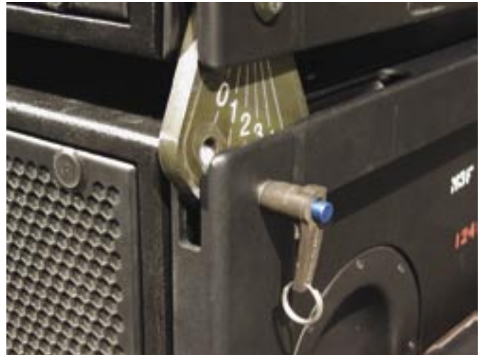
Figure 29. QRP fully inserted into 3° hole
